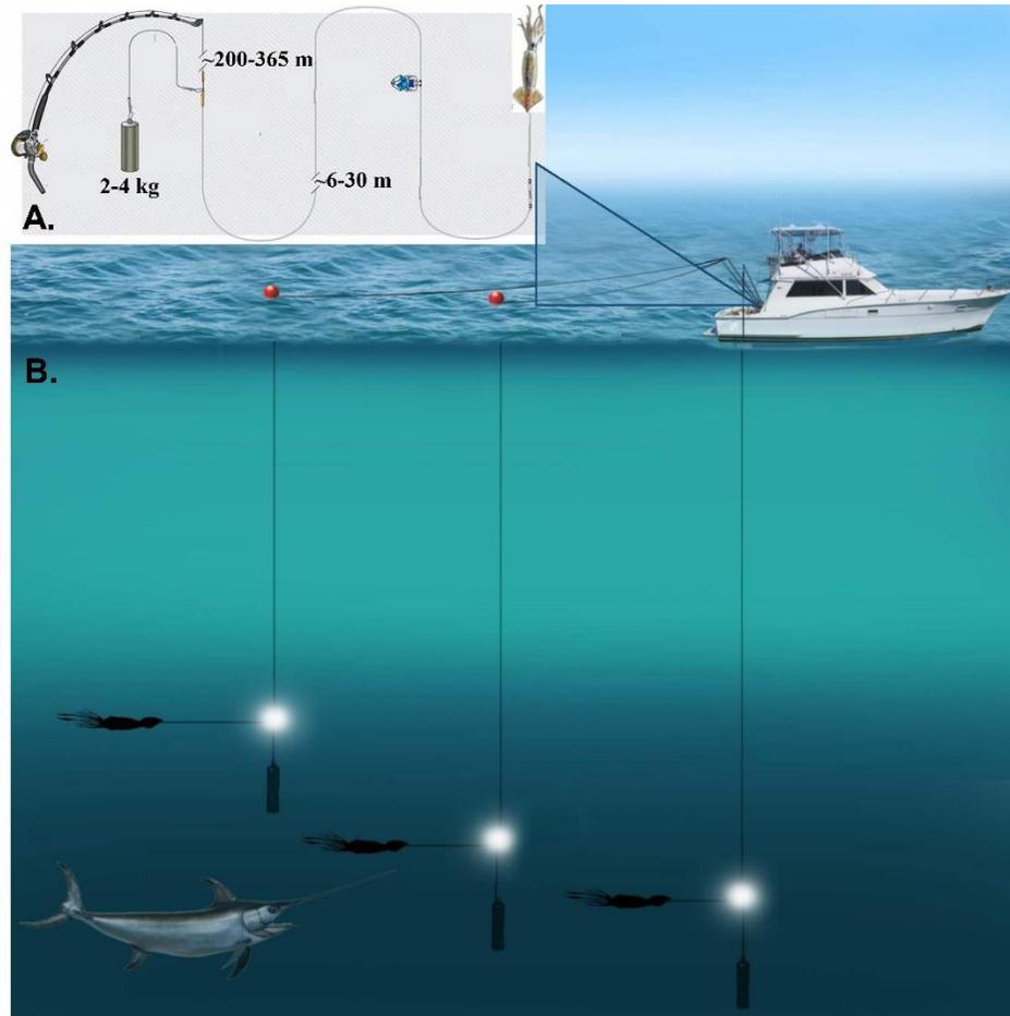
**Figure 2.** Depiction of a (A) common west-coast recreational swordfish gear setup using a heavily weighted vertical mainline and an illuminated gangion baited with jumbo squid and (B) standard configuration for targeting swordfish at depth during the daytime using multiple lines from a drifting vessel.
