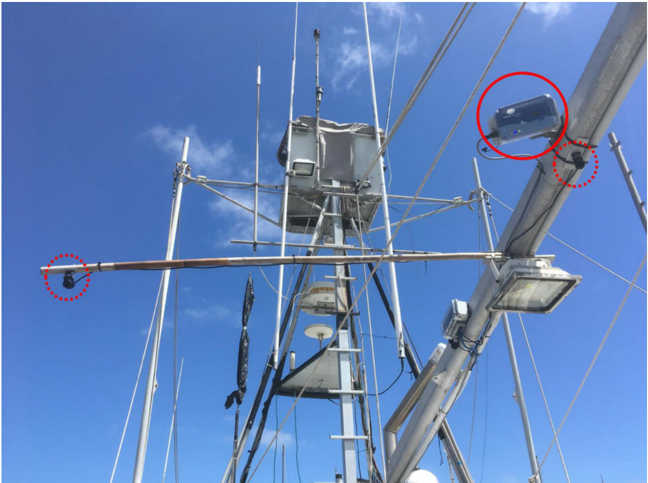
Figure 1.—Commercial swordfish vessel outfitted with two electronic monitoring (EM) platforms, including both a 1-camera system from Shellcatch Ltd (solid red circle) and a 2-camera system from Saltwater Inc (dashed red circle) during experimental deep-set fishing trials within the 2020–21 fishing seasons.
